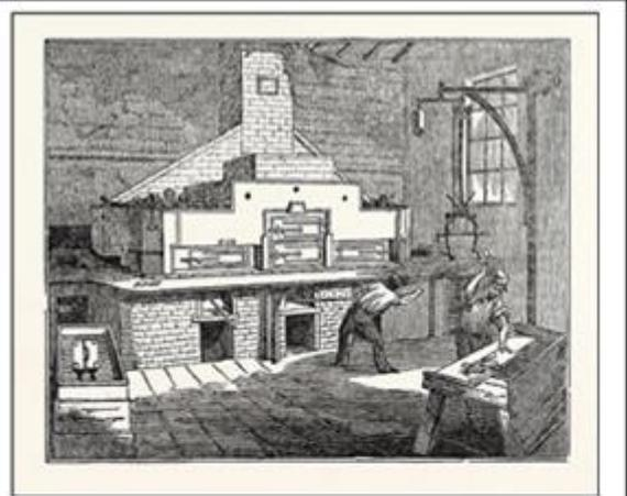
A Foundry is a factory that produces iron castings. Sand is placed in a refractory mold, a pattern is made of the object to be cast, and the pattern makes an impression in the sand. Molten iron from a furnace is poured from a crucible into the mold. The combination of a Foundry and a Machine Works enabled Cyrus Hall to keep his finishing operations running efficiently.
